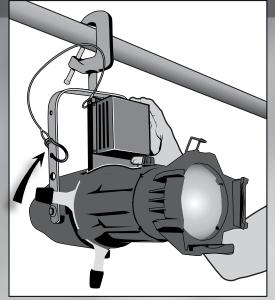
**2.** Be sure to attach the safety cable to lighting fixture.
